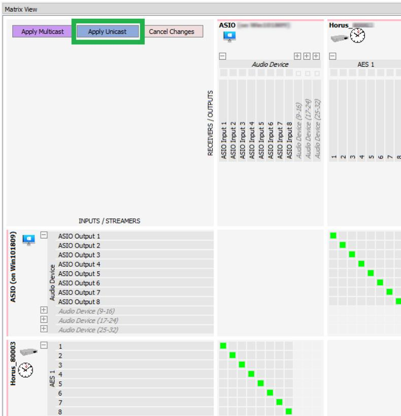
If only Apply Multicast is displayed, the device is not compatible with Unicast, please consult the device manual.
