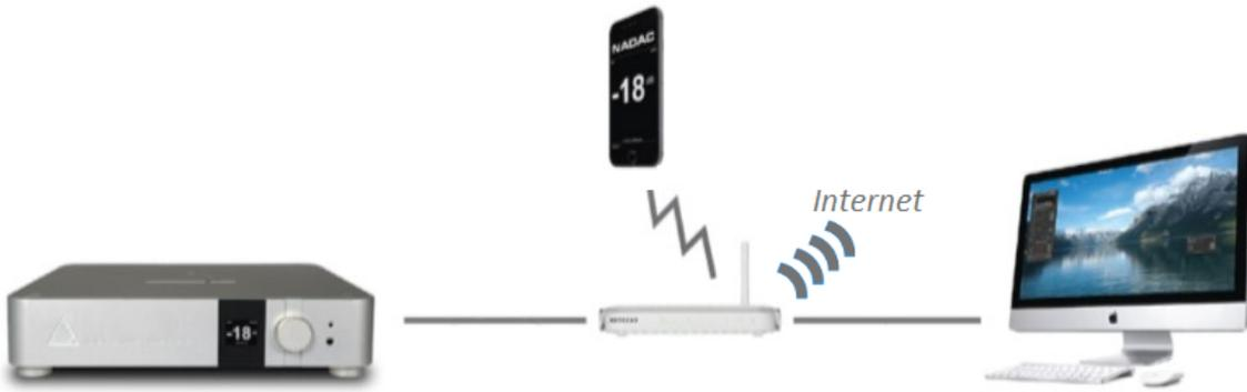
Configuration 2 : Connected to your network switch, connected to your home Router
