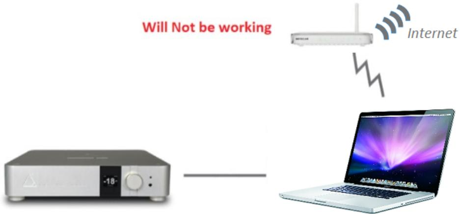
Wrong configuration : Connected to your network switch, without direct to your home Router.
